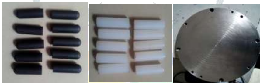
Figure2. Specimen of Teflon, PA6 pin specimen and SS410 Disk
