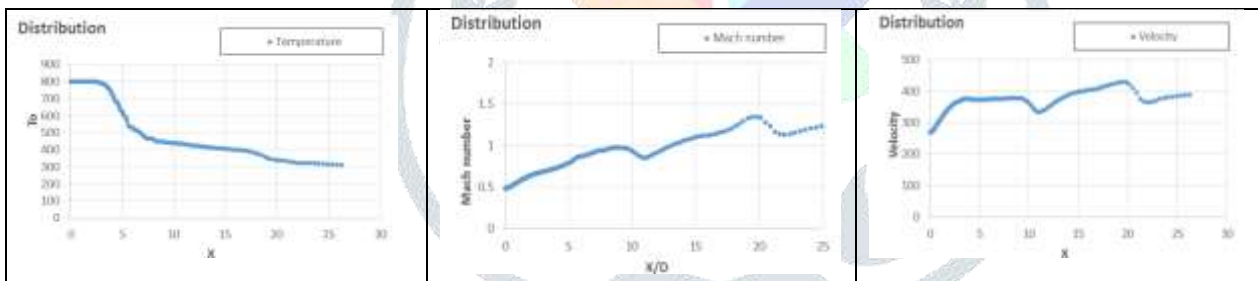
Fig 3.9- Distribution of Temperature, Mach no. and Velocity along the axis for baseline
