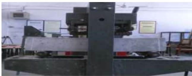
Fig. 6. Three -point loading machine
