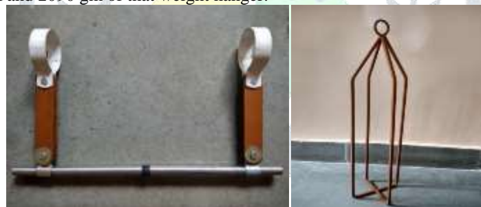
Figure: load frame and weight hanger manufactured as per required design arrangement.
