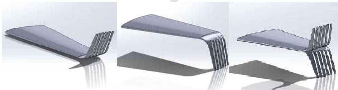
Fig 2.3: Feathered winglet on top, bottom view and both directions - 3D view
