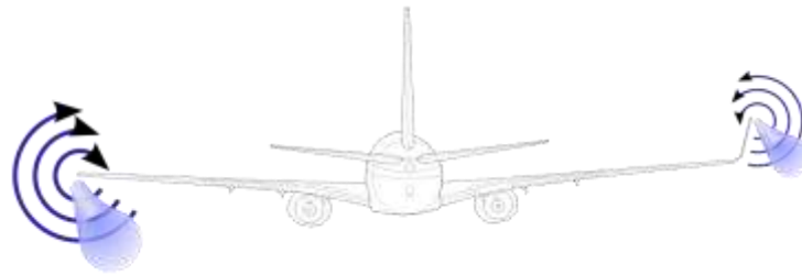
Fig 1.1: Effect of winglet on wingtip vortex
