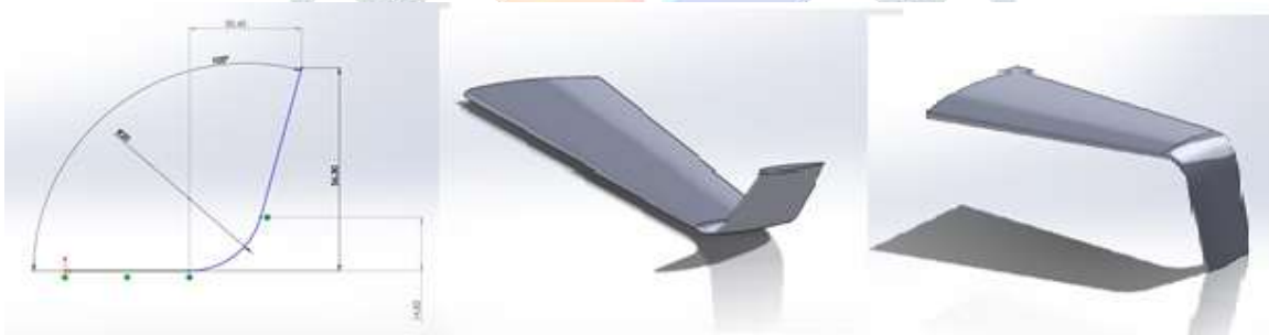
Fig 2.2: Details of the winglet shape, Baseline winglet towards the top and bottom
