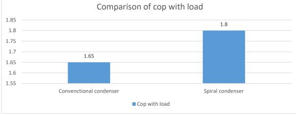
From fig.3.4, it is clear that coefficient of performance Cop and the modified system increased by10% when compared with normal system.
