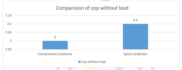
From fig. 3.3, it is clear that coefficient of performance Cop will be increased by 4.7% when compared with conventional system system.
