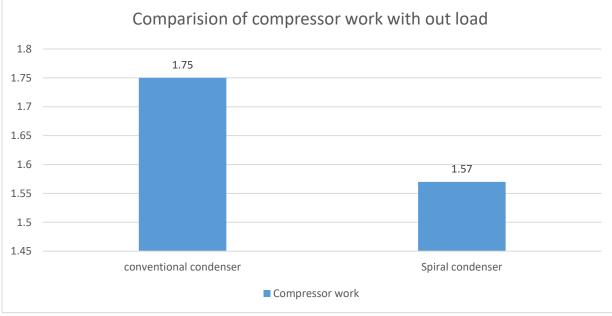
3.1.Comparison of compressor work at without load condition
