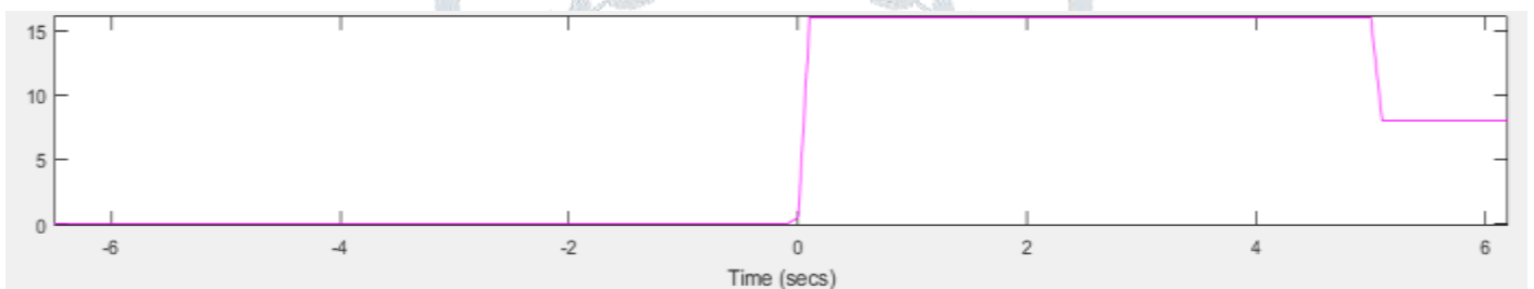
Figure 9 Load power consumption in constant current load in KW
