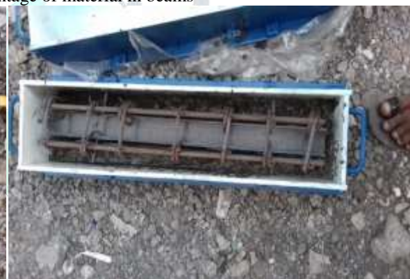
Fig -5: Casting of C-Channel GFRP beam
