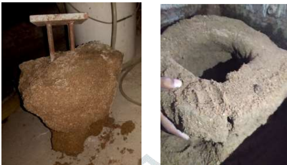
Figure 9: grouted foundation sand formations extracted after pile load test
