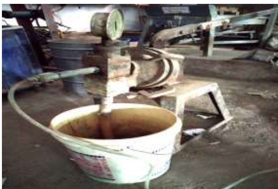
Figure 5: grout pump used in research
