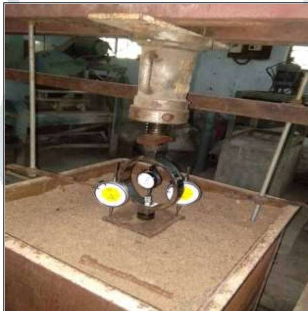
Figure 8: pile load test setup
