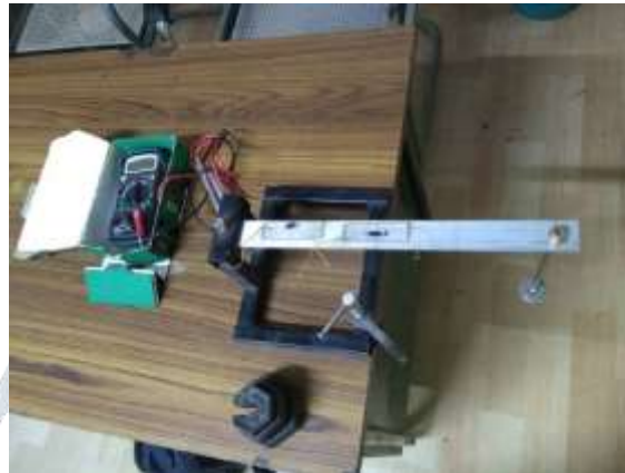
Figure 5 Bending test set up
