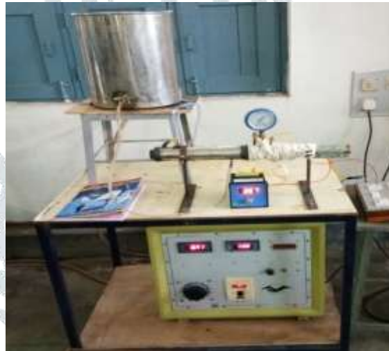
Fig.2: Experimental setup of the heat pipe
