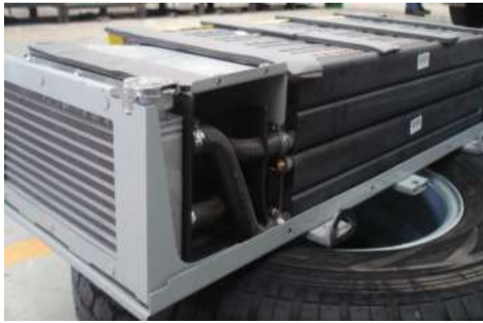
Figure 9. The NiMH HV battery cooling inlet & outlet
