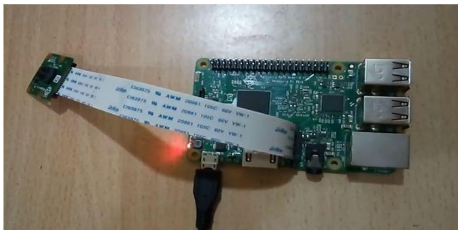
Figure 5.5: Hardware connection of PI cam with raspberry pi.
