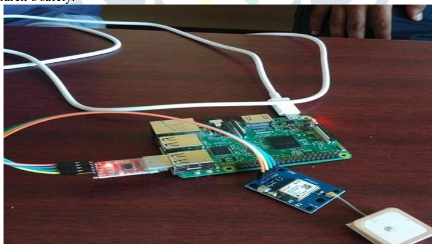
Figure 5.2: Hardware connection for location tracking.
