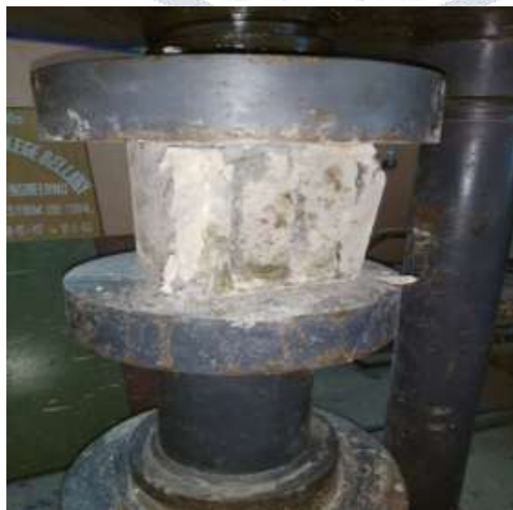
Fig 5.1 Compressive strength test on JFC cube
