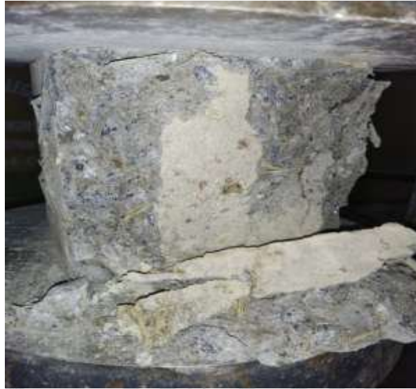
Fig 5.2 Failure of Jute fibre concrete cube
