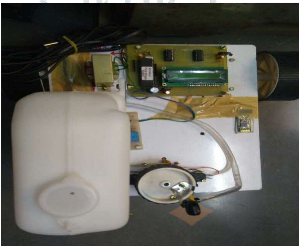
Fig.10. Complete Structure of Sprinkling and Weed cutting Module
