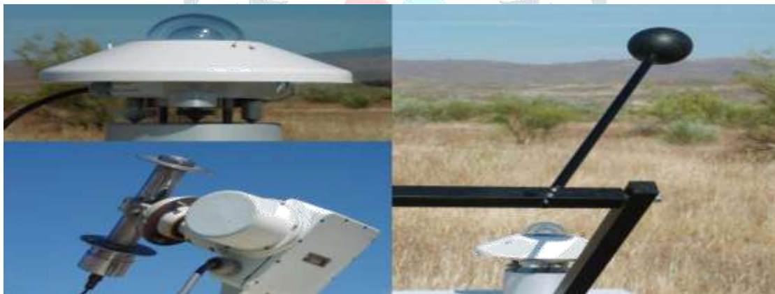
Fig 2.2 Pyranometer (left top), Two-axis tracked Pyrhemliometer (left bottom), Pyranometer with shading ball (right)
