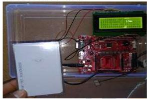
**Step2**: Read the RFID tag or ID card and compare with the address IDs stored in the server.
