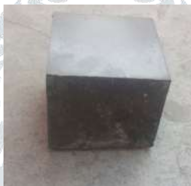
Fig. 2 As-cast Mg/SiC block
