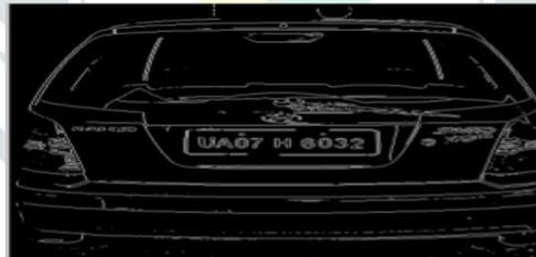
Figure. 6 Binary gradient image with sobel edge detector
