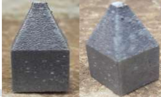
Aluminum alloy containing (0.8-1.2% magnesium, and 0.4-0.8% silicon)
