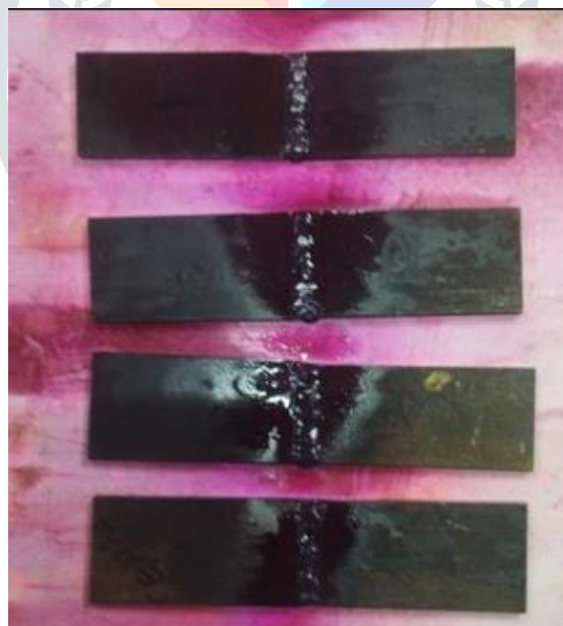
Penetrant of Welded Specimens
