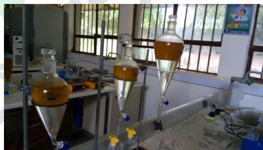
Fig 2. Washing of Biodiesel
