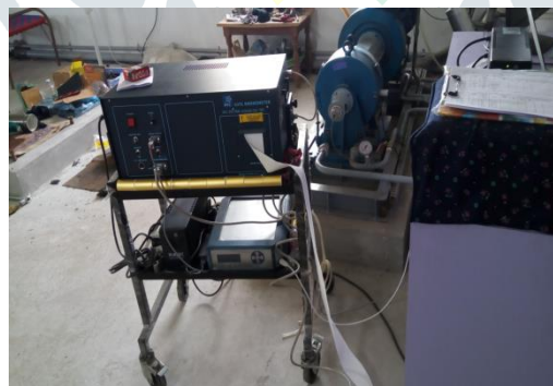
Fig 6. Emission measuring instruments (AVL 437C SMOKE METER, AVL DIGAS 444N)
