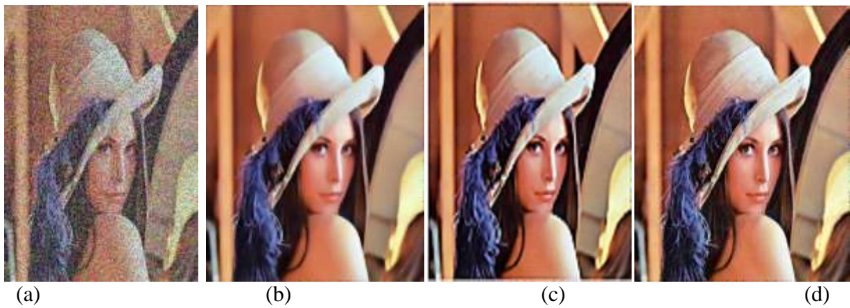
Figure 7: Denoising result of salt & pepper noise with noise variance \sigma=40 (a) Noisy image (b) output of DBMF (c) output of Ref [1] (d) output of Proposed Algorithm
