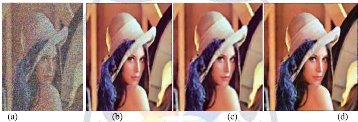
Figure 8: Denoising result of salt & pepper noise with noise variance \sigma=60 (a) Noisy image (b) output of DBMF (c) output of Ref [1] (d) output of Proposed Algorithm
