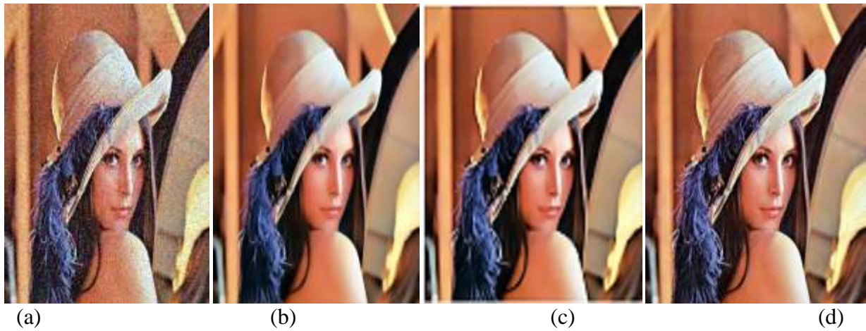
Figure 4: Denoising result of salt & pepper noise with noise variance \sigma=10 (a) Noisy image (b) output of DBMF (c) output of Ref [1] (d) output of Proposed Algorithm
