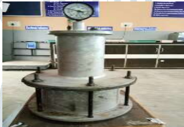
Fig:10 Test set up for water permeability of concrete
