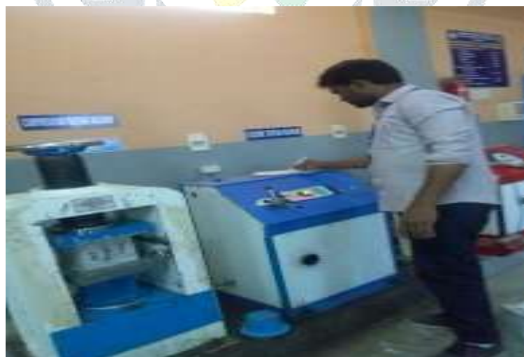
Fig:7 Compressive Strength test
