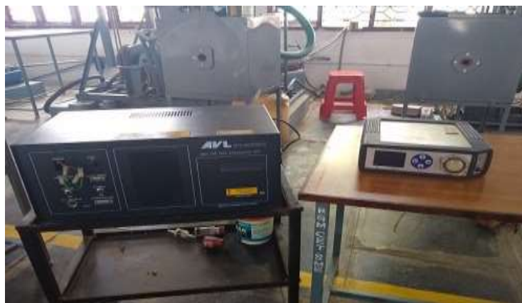
Fig4: AVL DIGAS-444 five gas analyser.
