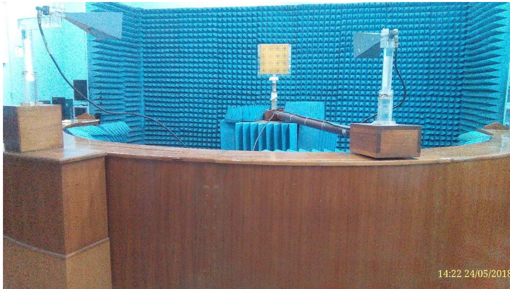
Fig.4 Photograph of the Arch method for scattering measurements of metallo-dielectric structures
