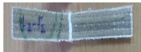
Fig.5: Flexural test specimen failure mode
