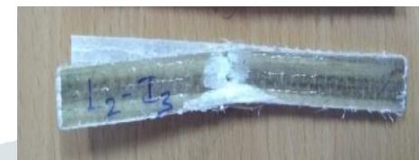
Fig.7: Impact test specimen failure mode
