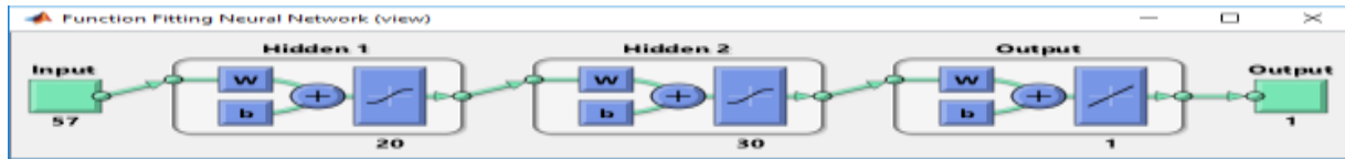
Fig : Neural Network with various size of layers having, 57 inputs and then a hidden layer of size 20 and then 30 and an output layer of size 1.
