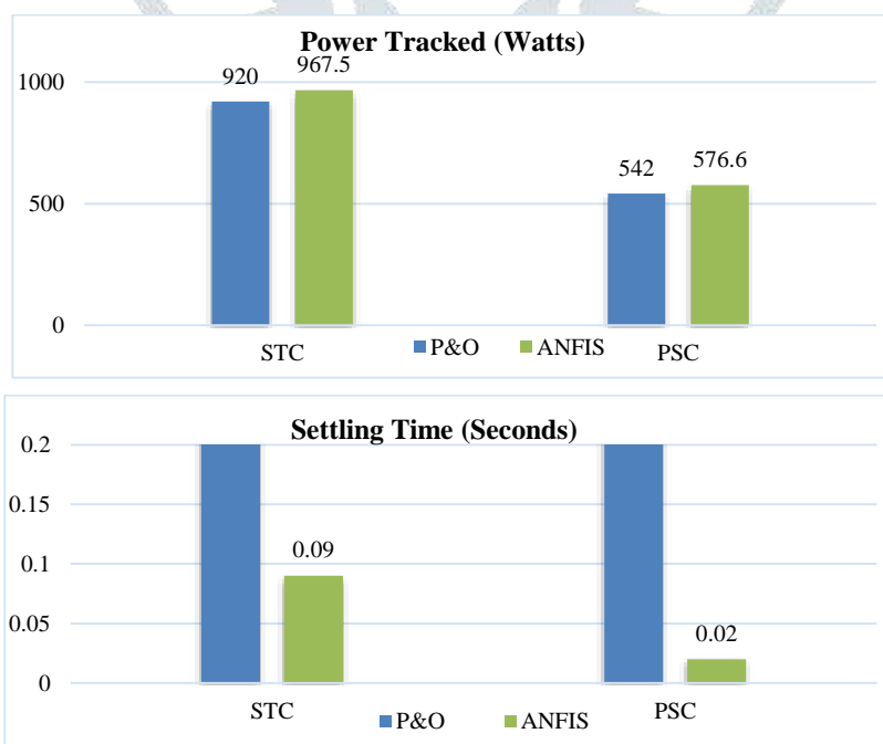
Fig.13 Comparison of power tracked and Settling Time of P&O and ANFIS under (a) STC (b) PSC
