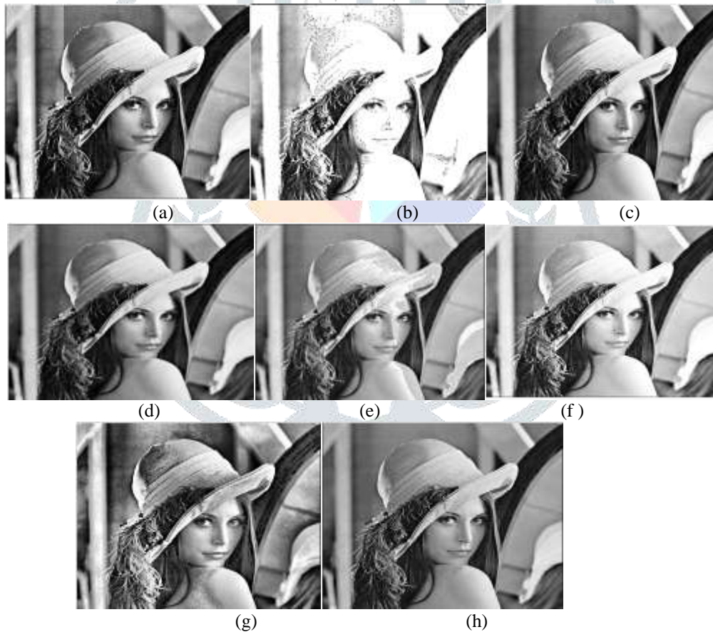
Fig 4.5 output obtained by applying different methods on sample natural image Fig.4.1 (e), (a) D-stretch and HE (b) BBHE (c) Histogram Equalization (d) DSIHE (e) Contrast stretching (f) Adaptive gamma correction with weighting distribution (g) CLAHE (h) Optimal gamma correction and weighted sum approach.
