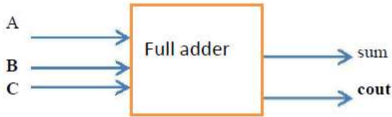
Figure.2 Block Diagram of Full Adder
