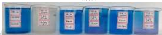
Photo 5: Effect of sunlight irradiation with respect to Dark condition and UV condition on photocatalytic degradation of DB 14 in 90 minutes.
