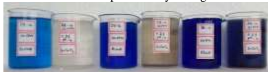
Photo 4: Effect of initial dye concentration on the photocatalytic degradation of DB 14 [ \text{SrCaO}_2 (urea) g/pH=0.2/4 and DB 14 = (30, 40 and 50) ppm]
