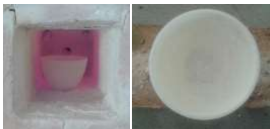
Photo 1: Synthesis of Nanoparticles by solution combustion method SrCaO 2 .
