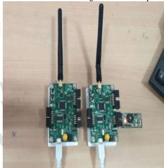
Figure 2. Setup of Communication Using C-Motes
