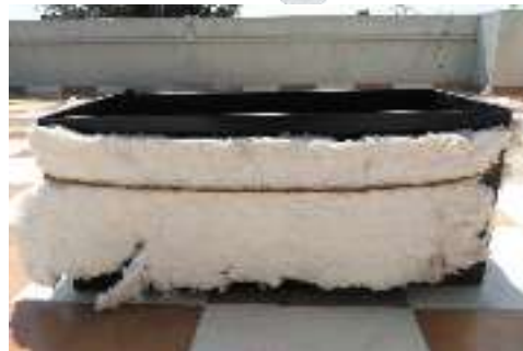
Fig.3 Experimental setup for solar still with coated with glass wool
