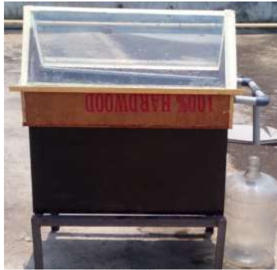
Fig.1 Experimental setup for Solar still with External Reflector
