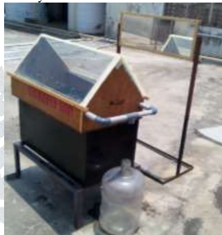
Fig.2 Experimental setup for Solarstill with External Reflector
