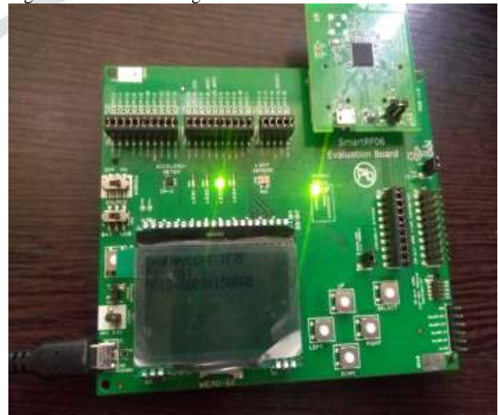
Figure 7.2.2: CC2538 Zigbee End Device Node
