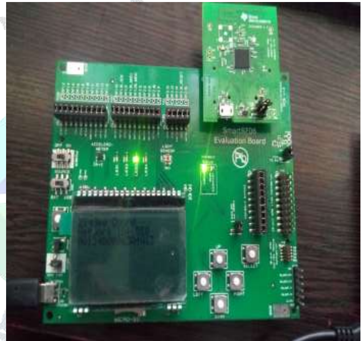
Figure 7.2.1: CC2538 Zigbee Coordinator Node
