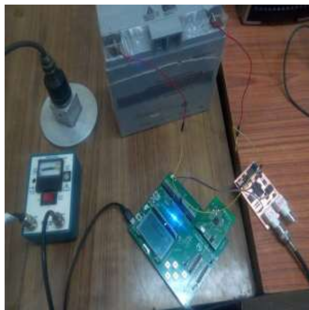
Figure 7.3.2: End node, Amplifier circuit with sensor
