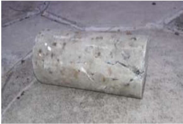
(b) Crack Pattern of Cylinder after Testing
