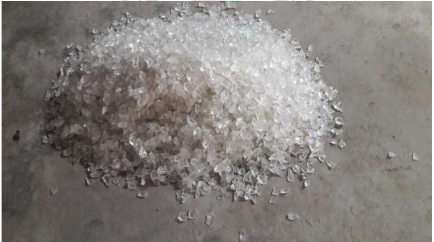
Fig 1: Recycled Waste Glass as Coarse Aggregate (RWG)
