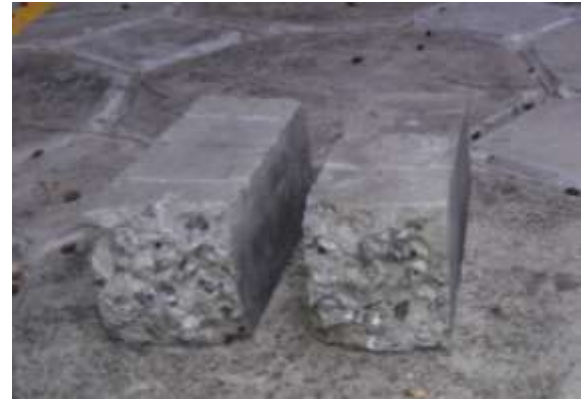
(c) Crack Pattern of Prism after Testing
