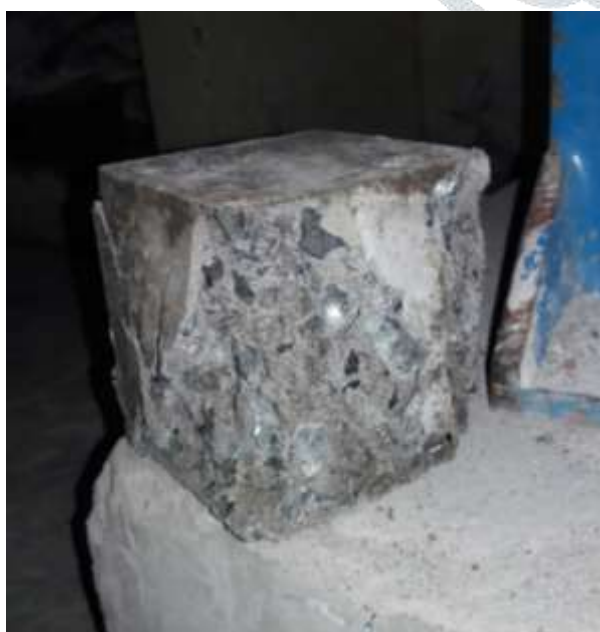
Fig 3: (a) Crack Pattern of Cubes after Testing
