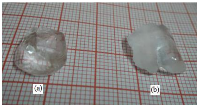
Fig.1. Harvested crystals of (a) undoped and (b) iodic acid doped LTLTA
