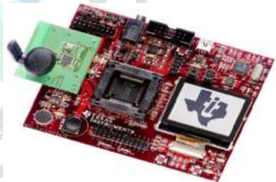
Figure 25: WSN node with MSP430F5438A and CC2520 RF Transceiver
