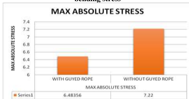
Max. Absolute Stress In above graph the max. absolute stress is 7.22 in without guyed rope zone. Max. Principal Stress
