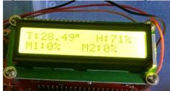
**Step3:** If temperature is more and soil moisture is low then the MCU switch ON the water motor.
