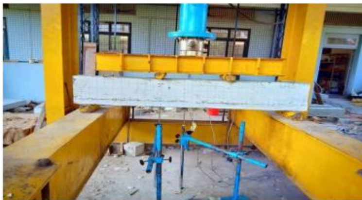
Experimental test set up for UHPFRC strengthened beam at tensile side
