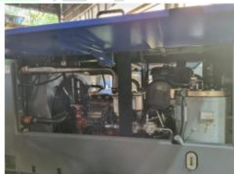
Oil injected screw air compressor package layout
