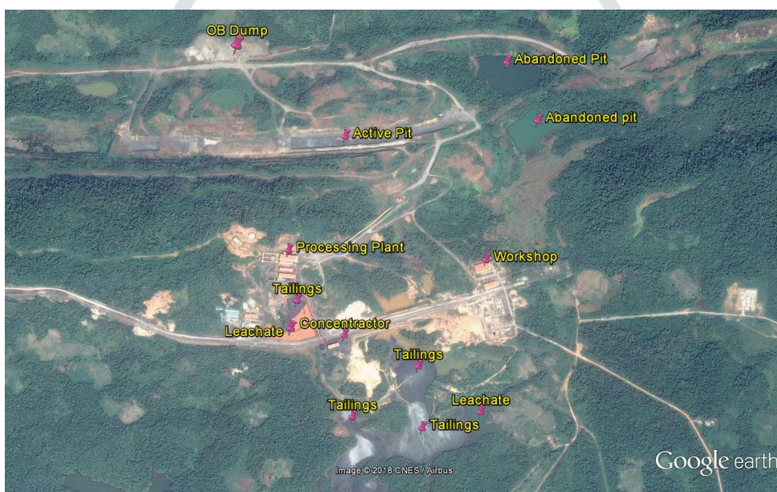
Fig. 3: Map of CUIOM showing sampling sites, abandoned mine pits, ob dump, and TSF and major mine facilities.
