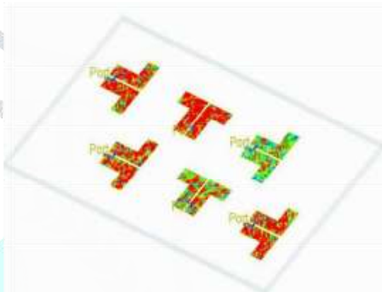
Figure 3.7 Simulated electric current distribution of printed dipole antenna in H-shaped configuration
