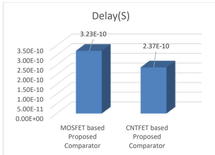
Figure 7. Delay comparison conventional proposed
