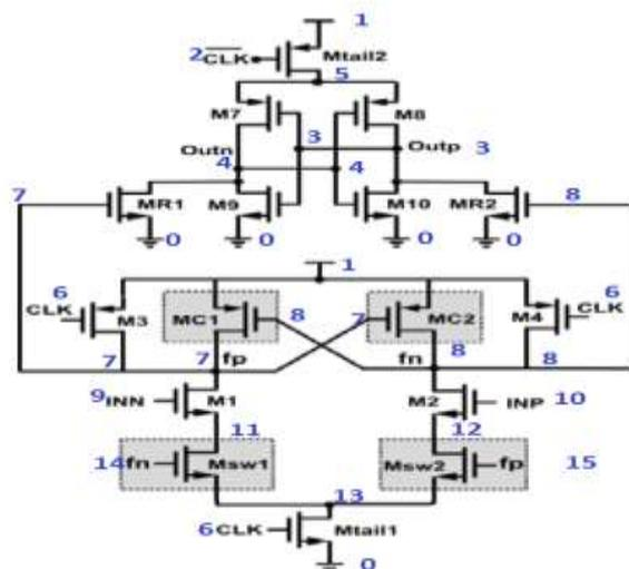
Figure 3. Proposed circuit using CNTFET
