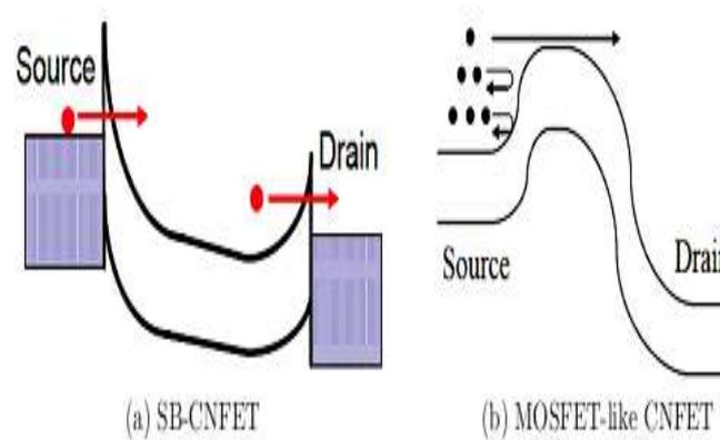
Figure 2. The energy band diagram for (a) SB-CNFET and (b) MOSFET-like CNFET
