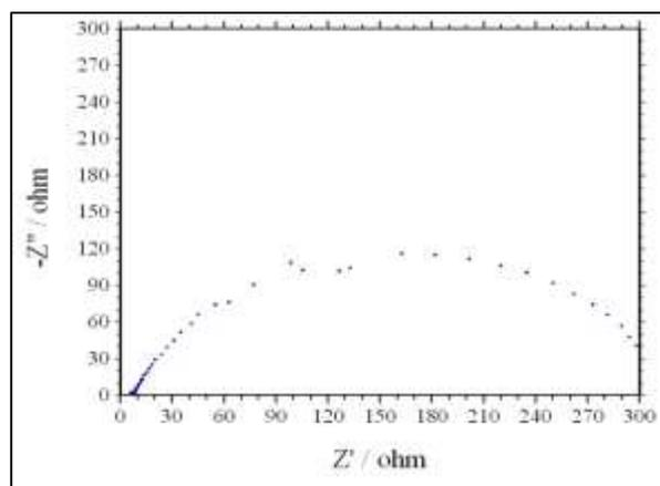
Fig. 5(a): Nyquist plot for brass in 0.1 M HNO<sub>3</sub>
