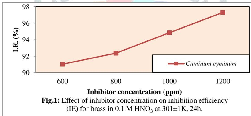
Fig.1: Effect of inhibitor concentration on inhibition efficiency (IE) for brass in 0.1 M  $HNO_3$  at  $301 \pm 1$  K, 24h.
