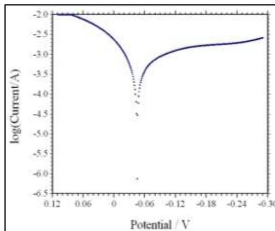
**Fig. 4(a):** Potentiodynamic polarization curve for brass in 0.1 M HNO<sub>3</sub>
