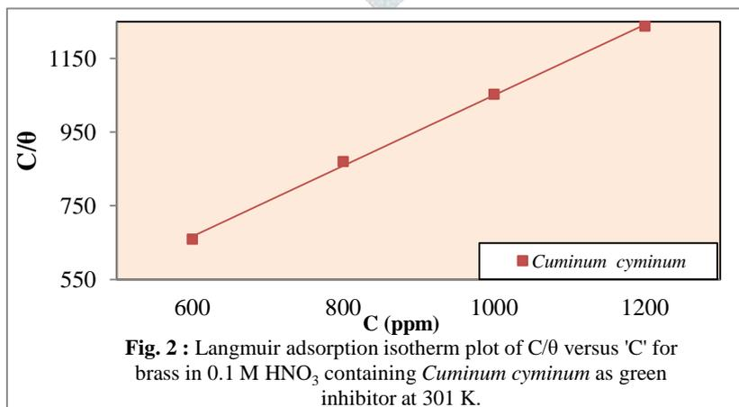
Fig. 2 : Langmuir adsorption isotherm plot of  $C/\theta$  versus 'C' for brass in 0.1 M  $HNO_3$  containing *Cuminum cyminum* as green inhibitor at 301 K.
