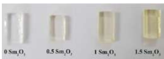
Fig. 1 Glasses with different concentrations of \text{Sm}^{3+} ion doped NPABS glasses
