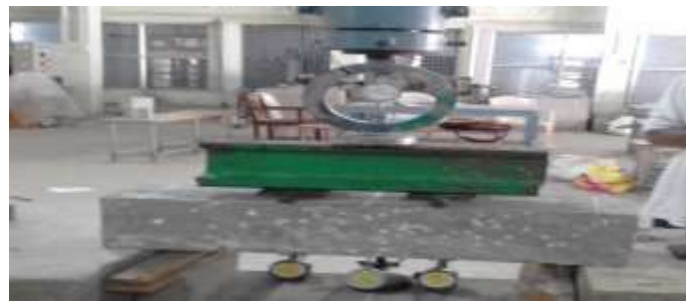
Fig.4.1: Test setup for Flexure strength of beam
