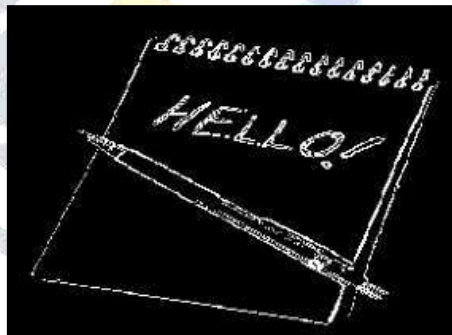
Fig 7.b.Sobel edge detection image
