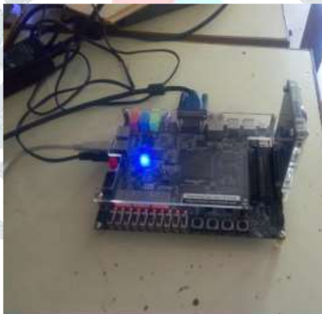
Fig 6.Altera Cyclone V DE1 SoC development board interface with TRDB-D5M camera
