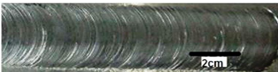
Fig 2 Surface morphologies of weld without defects
